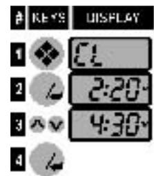
The time of day function allows the user to set the internal clock of the power unit to the current time. The unit will keep time for  $\pm 48$  hours in case of power failure. The following is the procedure to set or modify the time of day.
